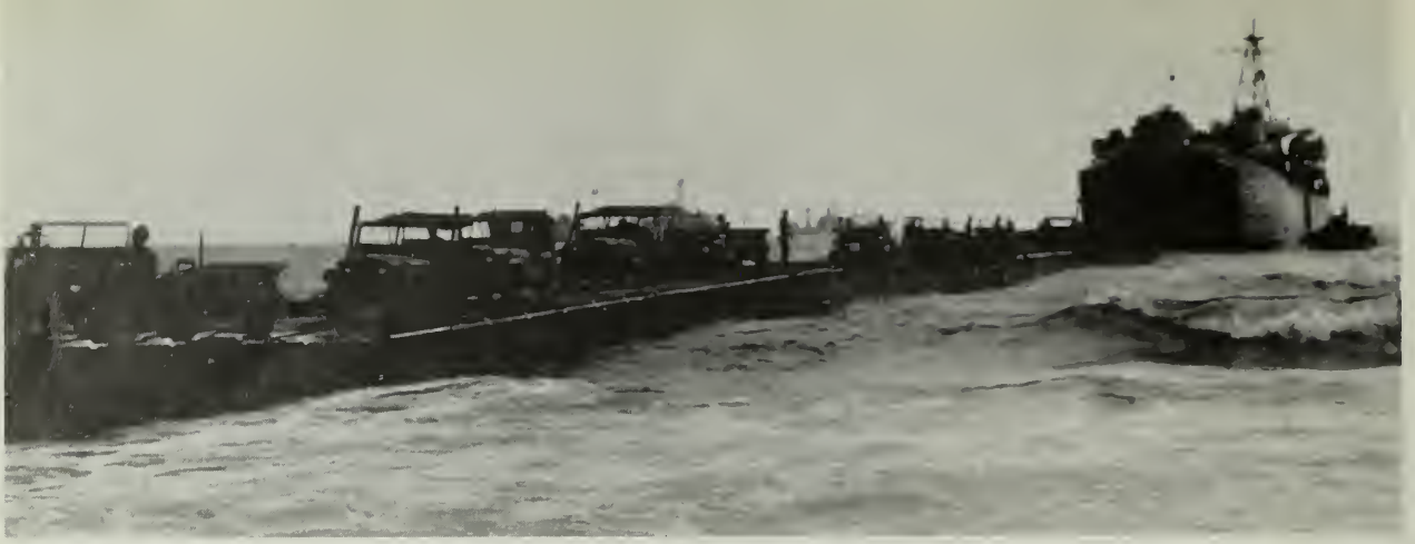
TANK LANDING ship puts support vehicles and equipment ashore by use of pontoon causeway leading to the beach.
